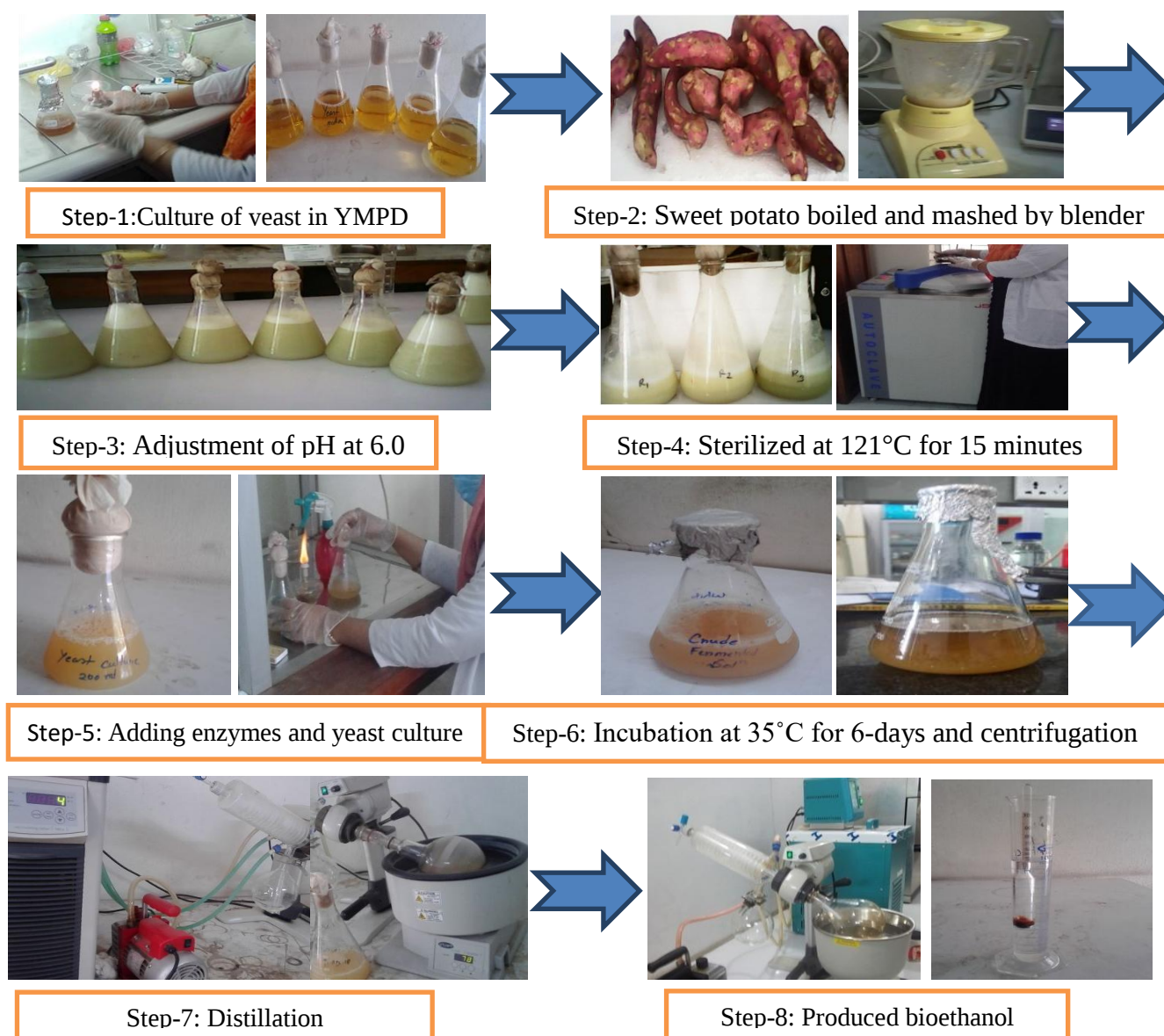
Fig. 1. Flow-chart of bioethanol production from sweet potato
